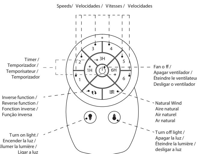
**Note:** To change the light tone press button " " and the light will turn on, press " " to turn it off and press " " again and the light will turn on in a different tone.
