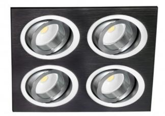
Cut out (mm): 165x165 mm. Weight (Kg): 0.57 Material: Aluminium Finish: Black - Stainless IP Rating: 20 Lamp holder: G5.3 Voltage (V): 230 IEC protection: Class III Tilting Angle: 30° Dimensions (mm): 175x175x25 Pcs / Pack: 1
