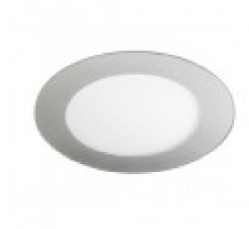
Cut out (mm): Ø155 Weight (Kg): 0.45 LED type: LED SMD Power (W): 12 Brightness (Lm): 970 Light temperature (K): 4000 Beam angle: 120° ON/OFF: 10.000 Voltage (V): 230 Dimensions (mm): 173x22 Pcs / Pack: 1
