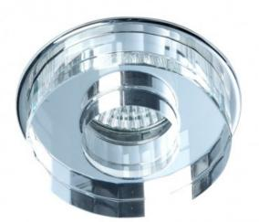
Shape: Round Height (mm): 40 mm Length (mm): 90 Width (mm): 90 Cut out (mm): Ø70 Weight (Kg): 0.505 Material: Aluminium and K9 optical glass IP Rating: 20 IEC protection: Class III Lampholder included: 5.3 Pcs / Pack: 1
