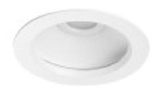
Cut out (mm): Ø160 Material: Aluminium and glass IP Rating: 20 LED type: LED Power (W): 12 Brightness (Lm): 900 Lifetime (h): 25.000 Voltage (V): 220-240 Frequency (Hz): 50 IEC protection: Class II Tilting Angle: 120° Dimensions (mm): Ø 175
